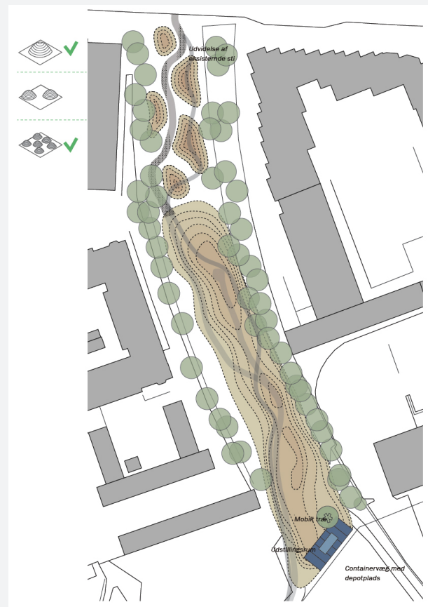
Figure 4.4 Modelling of temporary soil storage in function of local needs (City of Copenhagen)
