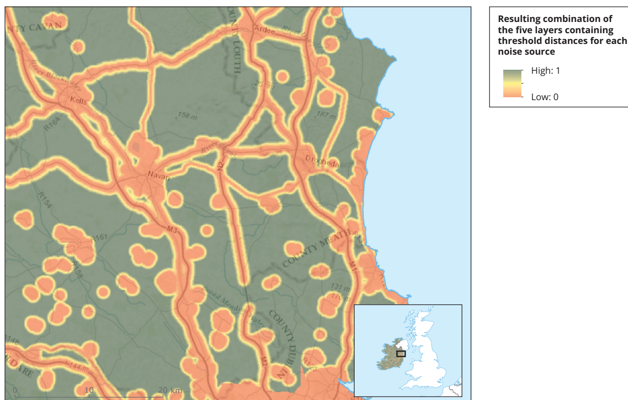
Figure A2.2 Example of the combination of five layers containing threshold distances for each noise source
