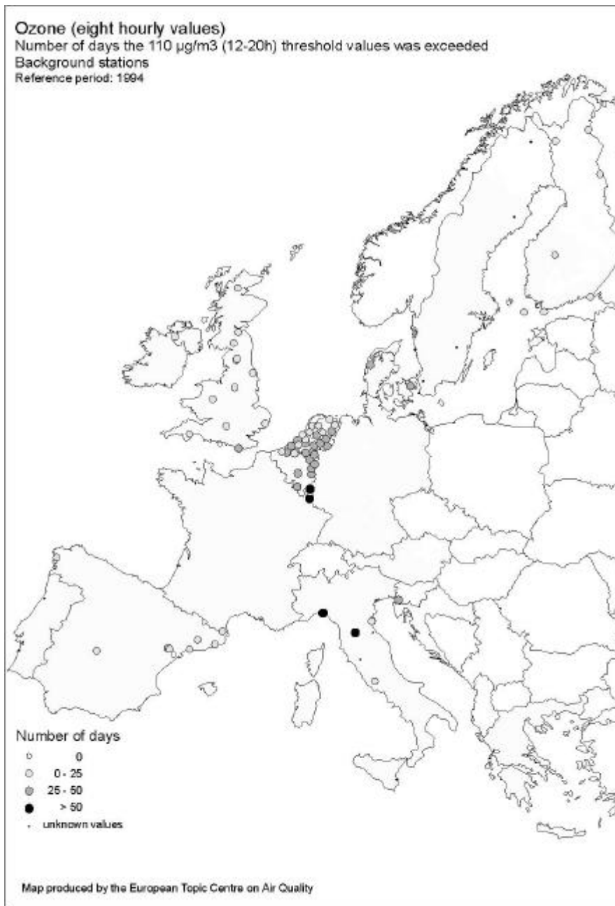
Figure 6.53: Number of exceedances of the threshold value for protection of human health ( 110 \mu\text{g}/\text{m}^3 for eight hourly values) observed at background stations; calendar year 1994; eight hourly averaged values for the period 12.00-20.00.
