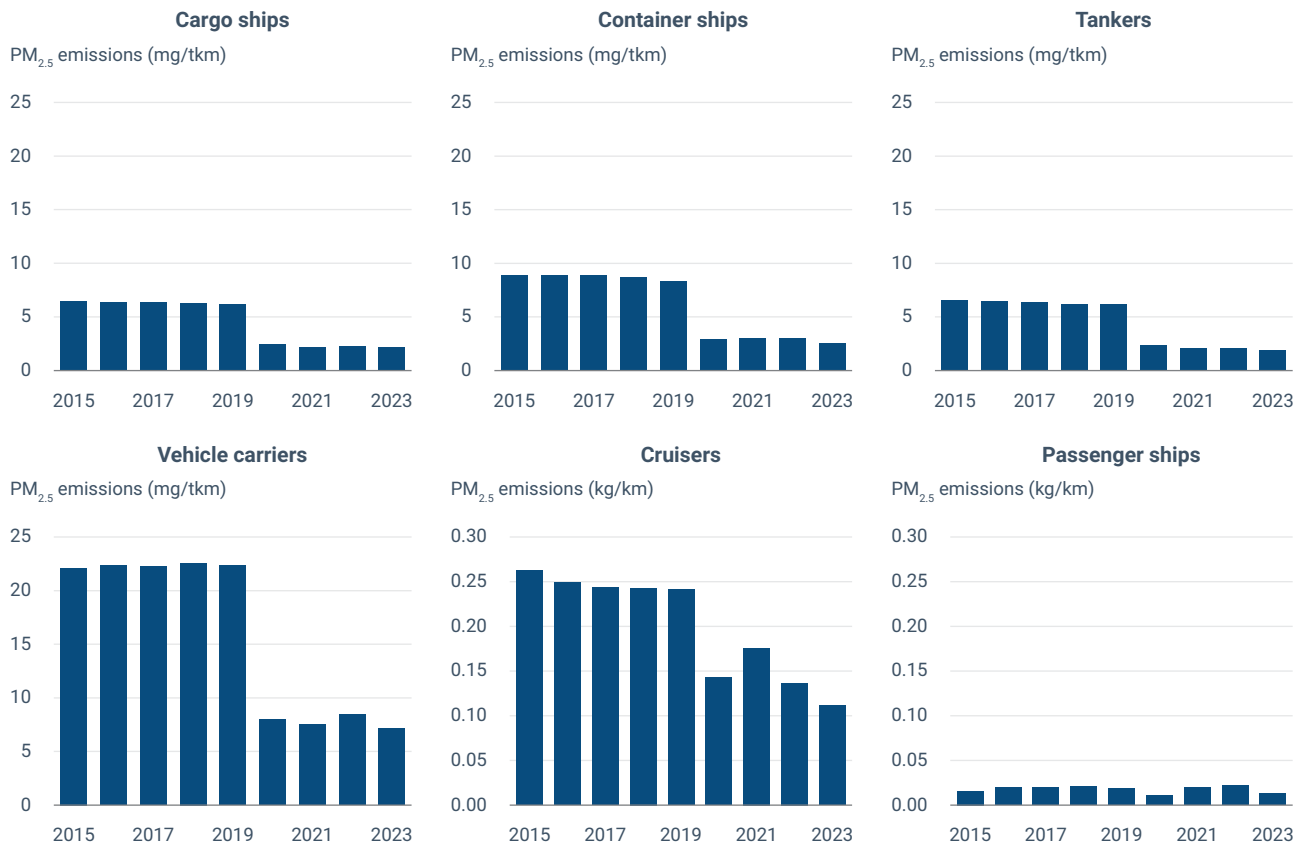
Figure 2.15 PM 2.5 specific emissions from selected freight and passenger ship types in the EU-27
