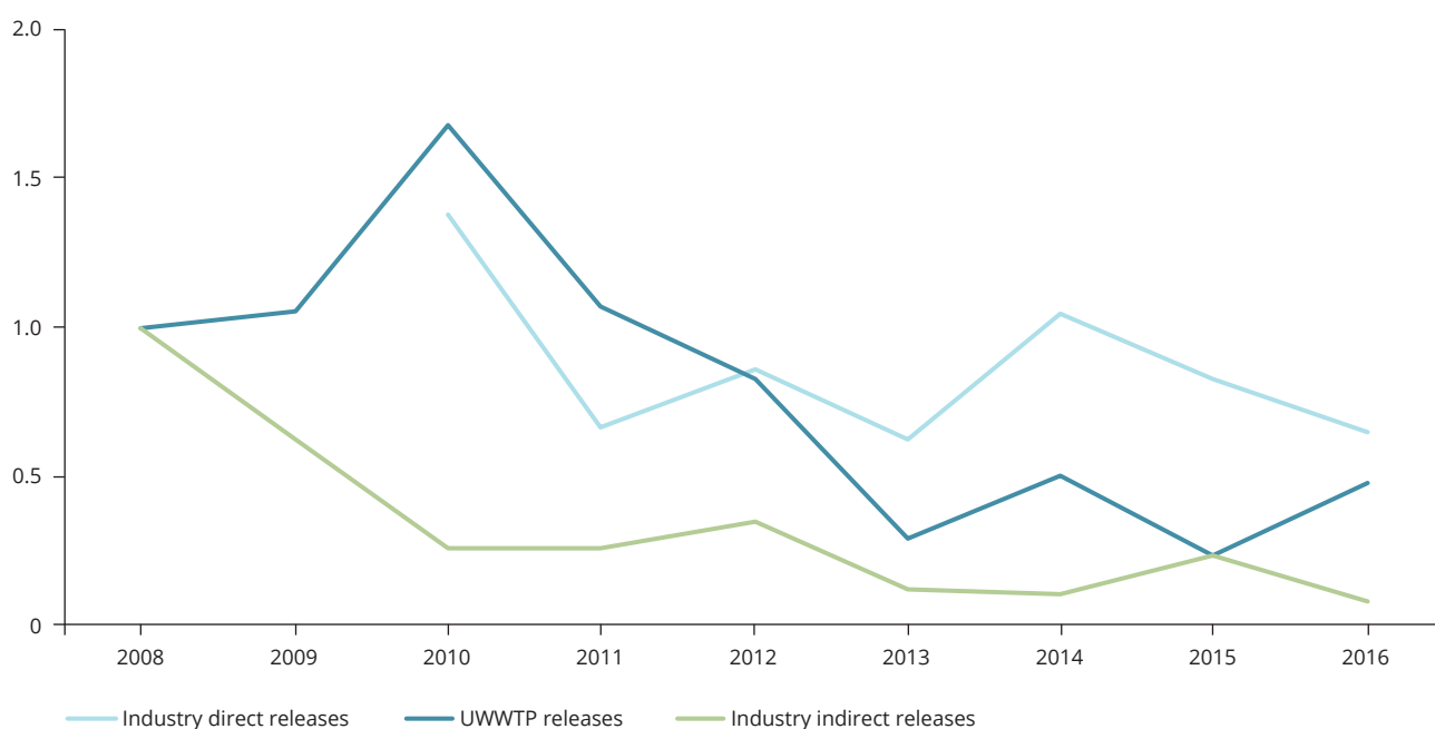
Figure 2.21 Trends over time in emissions of chlorinated organic substances from industry and UWWTPs, expressed as eco-toxicity, 2008-2016
