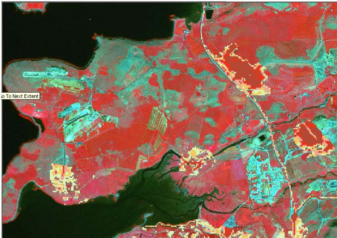
Fig. 5a. (See Fig. 5b for comparison) Soil sealing dataset on top of a SPOT-5 image showing misclassification on construction sites (the two red spots in the right half of the image). The soil sealing spot in the centre of the image is a mixture of a sport and leisure area and semi-natural vegetation and the spot in the left half is simply sparsely vegetated.
