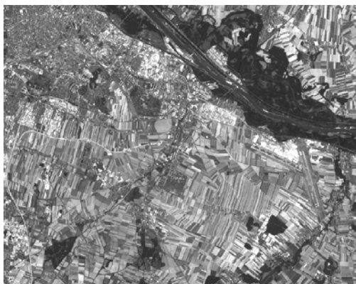
SPOT-4 satellite image over Vienna / Austria (green band; 20m resolution)
